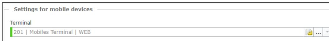
To activate the transfer of GPS coordinates for ZEUS®X mobile, go to ‘Settings → Patterns → Terminals → Booking action’. Open the **Booking action** tab and select the corresponding option from the drop-down menu. If **Required** is selected, bookings *without* GPS coordinates are listed in the Dashboard widget **Exceptions** and must be approved before being processed.
